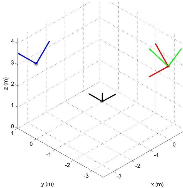
FIGURE 1. The bistatic scattering scene. The transmitter, receiver and scattering points are shown in blue, red and black respectively. The polarization rotation due to specular scattering is  $69^\circ$  and represented in green.
