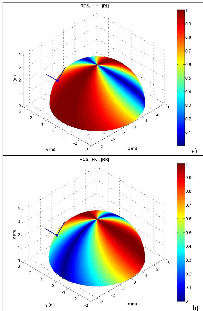
FIGURE 3. Receiver Bistatic RCS datadome of a sphere in the physical optics regime showing linear and circular polarization basis combinations. The transmitter is located at azimuth =  $0^\circ$  and elevation =  $45^\circ$ , whereas the receiver is swept over the datadome hemisphere.
