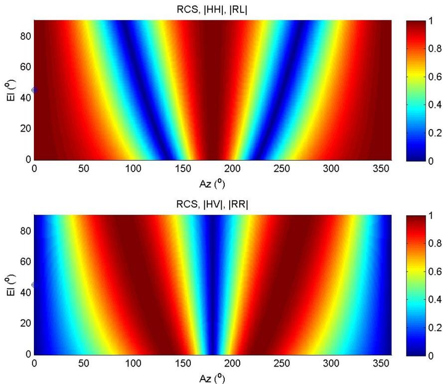
FIGURE 2. Bistatic RCS of a sphere in the physical optics regime showing linear and circular polarization basis combinations. The transmitter is located at azimuth =  $0$  and elevation =  $45^\circ$ , whereas the receiver is swept over the datadome hemisphere.
