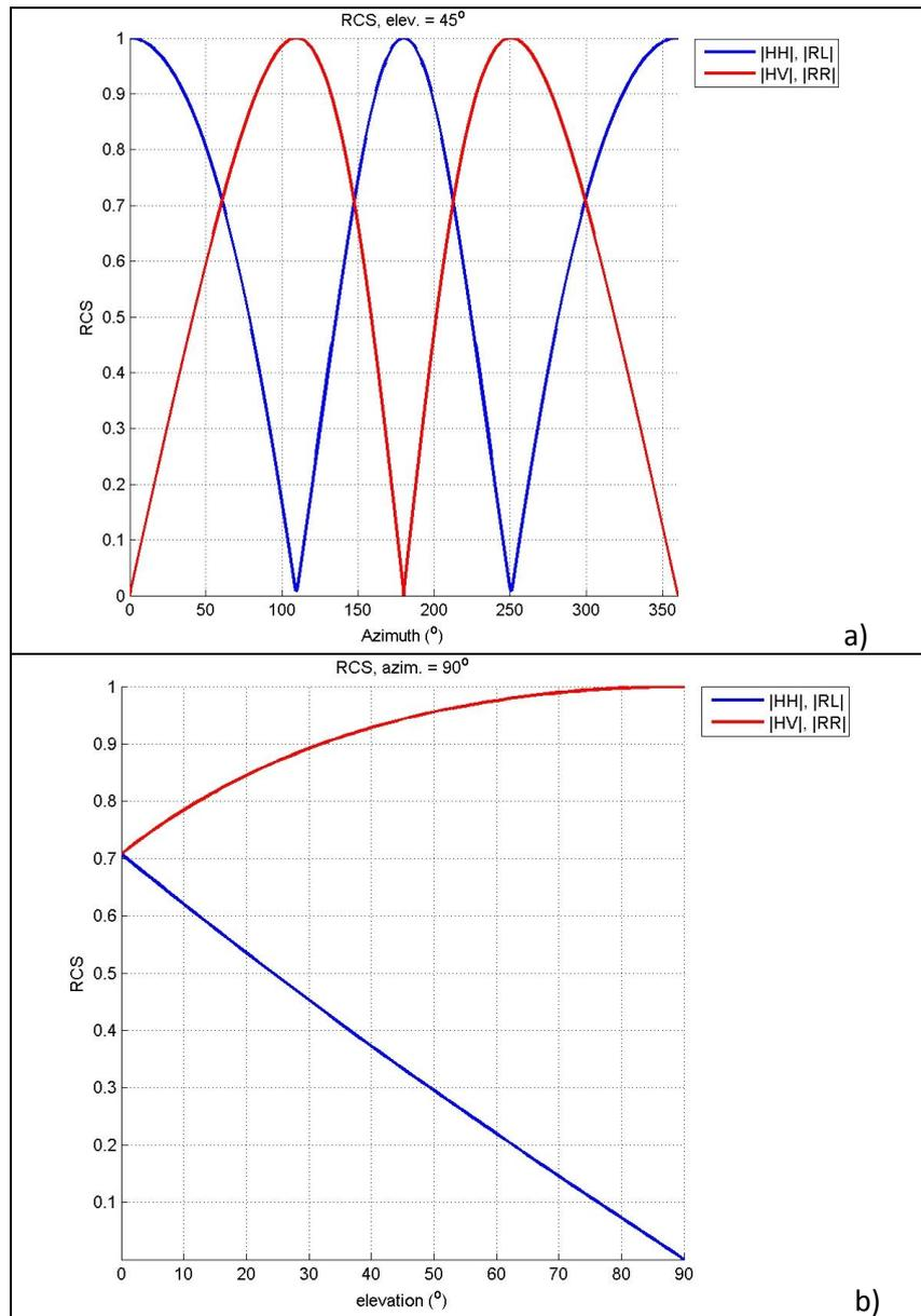
FIGURE 4. Graphs showing receiver azimuth or elevation cuts through the bistatic RCS polarization datadomes presented in Figures 2 and 3. (a) presents azimuth cuts where the elevation angle is fixed at  $45^\circ$ . (b) presents elevation cuts where the receiver azimuth angle is fixed at  $90^\circ$  (b). In both cases the transmitter position is fixed at  $0^\circ$  azimuth angle and  $45^\circ$  grazing angle.
