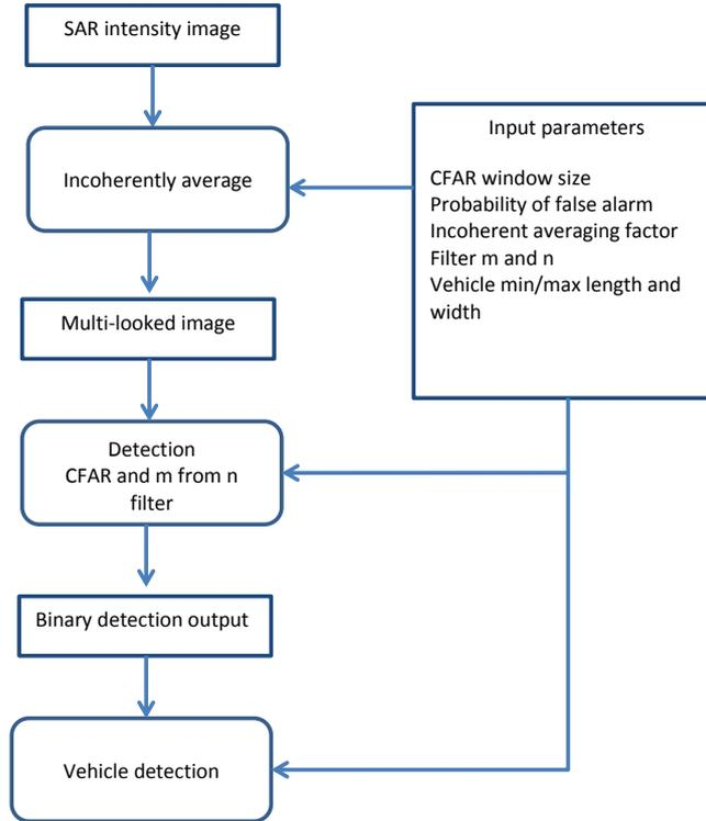
FIGURE 1. Vehicle detection algorithm
