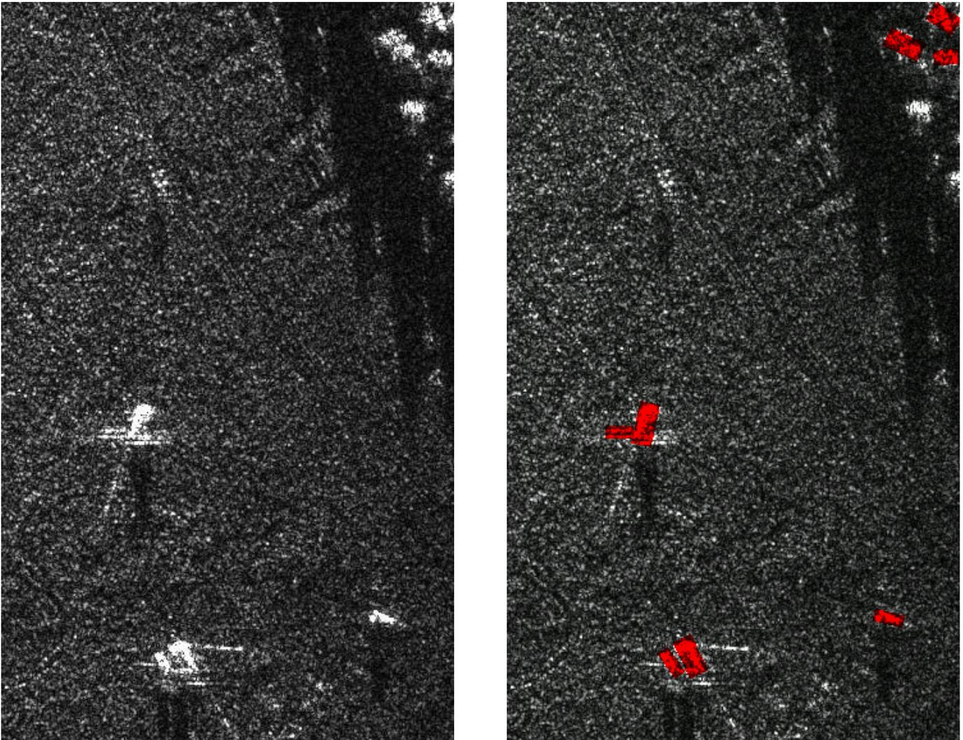
FIGURE 8. Vehicle detection results. Left: Original SAR image, right: SAR image with vehicle detections overlaid
