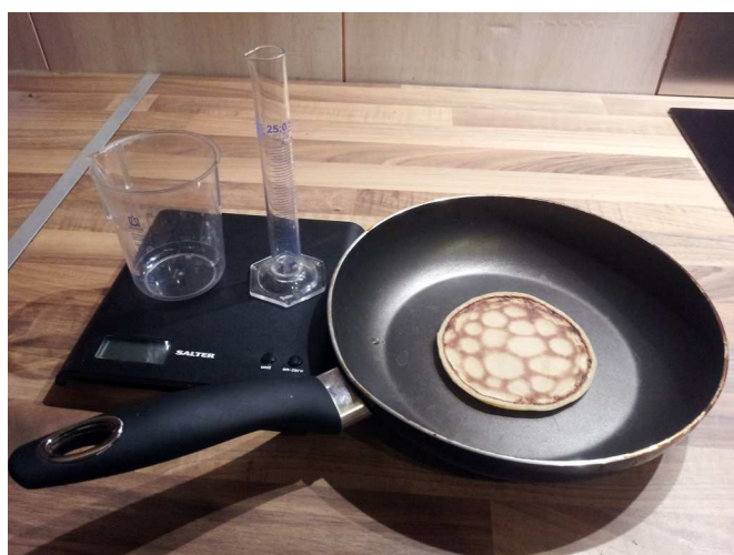
Figure 2: Photograph showing the kitchen study. The apparatus consisted of a frying pan, a 250 ml beaker, a 25 ml graduated cylinder and kitchen scales.
