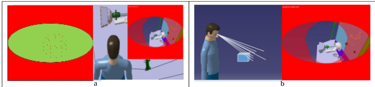
Figure 5.(a) Feature points in maintenance vision distribution and Delmia verification diagram (b) Visual occlusion evaluation effect and Delmia verification diagram
