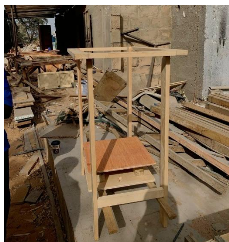
Harmonograph building in progress at Lycée Limamoulaye in Senegal
